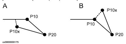
In both examples, when restarting the program the robot continues from the new P10 (that is now the same as P10x) directly to P20 without returning to the previous planned path (via the old P10).
